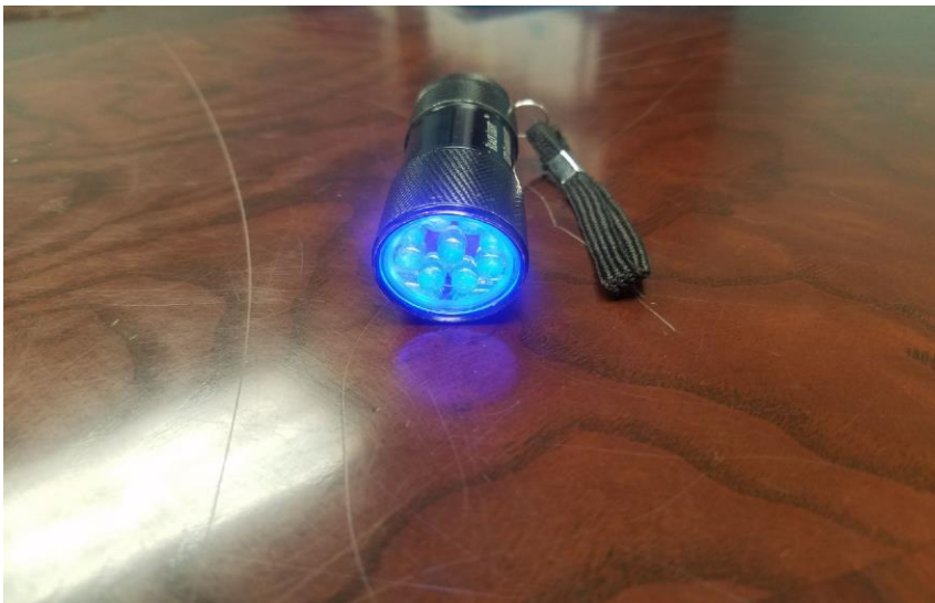
Figure 2. Blacklight flashlight used by supervisors at the subject hospital to check on the existence of marks made at discharged rooms using translucent marker. Absence of mark after the discharged room cleaning indicates thorough cleaning.
