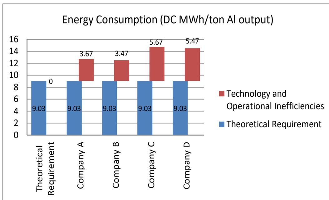
*Figure 44.* Energy efficiency of all four companies studied compared with the technical requirement.
