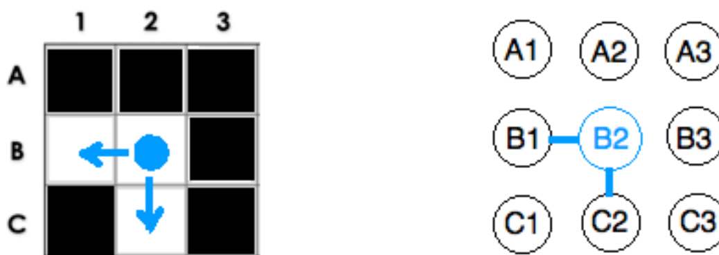
Low density (high occlusion) grid map on left, with corresponding graph representation on right. Note how only grid cells (vertices) B1 and C2 are reachable from B2.
