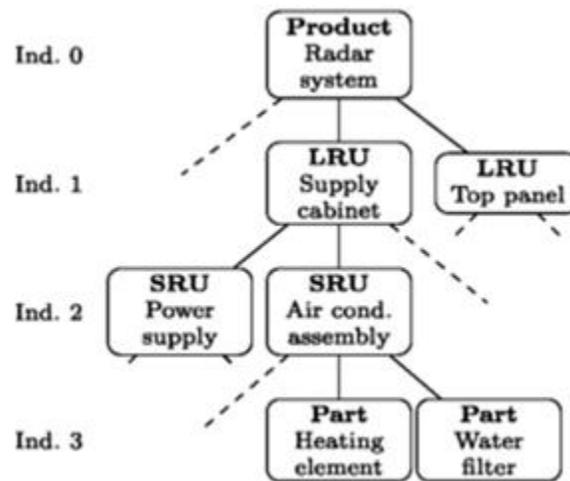
*Figure 1.* Radar system indenture product structure. Adopted from “An Approximate Approach for the Joint Problem of Level of Repair Analysis and Spare Parts Stocking,” by R. J. Basten, M. C. Van der Heijden, J. M. J. Schutten, and E. Kutanoglu, 2015, *Annals of Operations Research*, 224, p. 122. Copyright 2012 by Springer Science & Business Media, LLC. Reprinted with permission (Appendix H).
