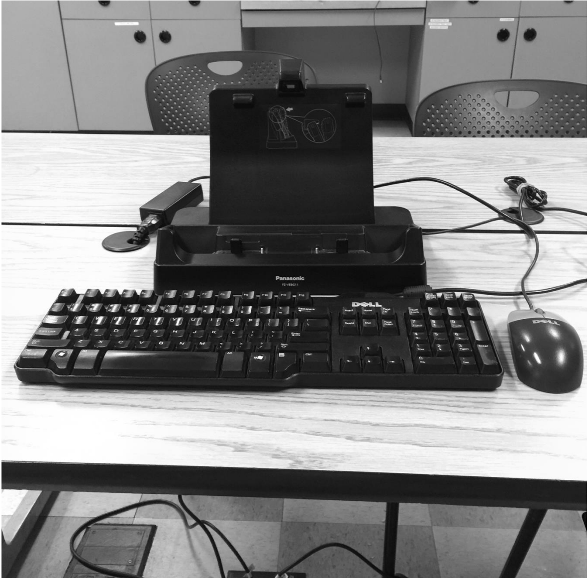
Figure 1. An example of a tablet docking unit inside a GPD station.
