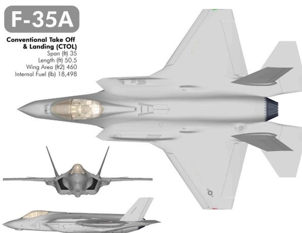
*Figure 1.* F-35A conventional takeoff & landing (CTOL). From “F-35 Variants,” by F-35 Lightning II Program, n.d., retrieved from [http://www.jsf.mil/f35/f35\\_variants.htm](http://www.jsf.mil/f35/f35_variants.htm)
