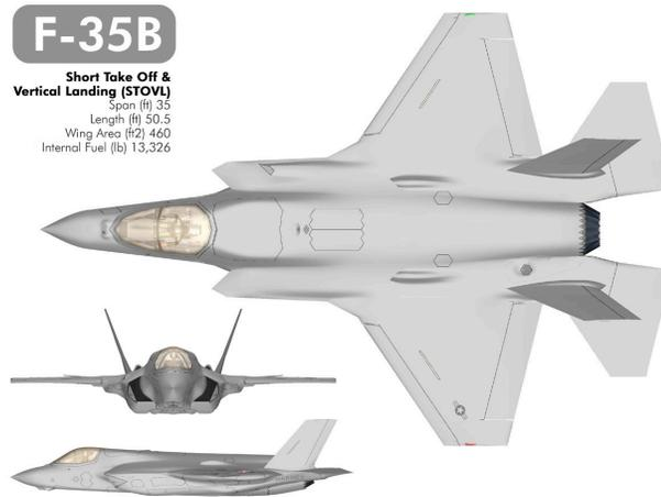
*Figure 2.* F-35B short takeoff & vertical landing (STOVL). From “F-35 Variants,” by F-35 Lightning II Program, n.d., retrieved from [http://www.jsf.mil/f35/f35\\_variants.htm](http://www.jsf.mil/f35/f35_variants.htm)
