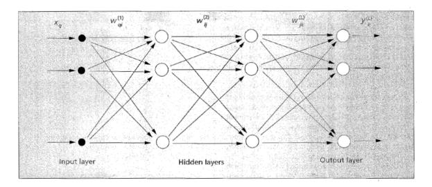
*Figure 7*. Model Feedforward Neural Network (FFNN) by A. Jann and J. Mao (1996). Artificial Neural Networks: a Tutorial, *Institute of Electrical and Electronics Engineers*, 194-212.
