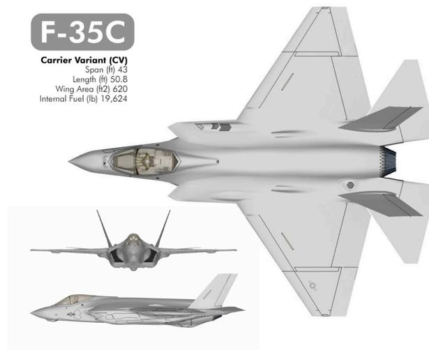
*Figure 3.* F-35C carrier variant (CV). From “F-35 Variants,” by F-35 Lightning II Program, n.d., retrieved from [http://www.jsf.mil/f35/f35\\_variants.htm](http://www.jsf.mil/f35/f35_variants.htm)
